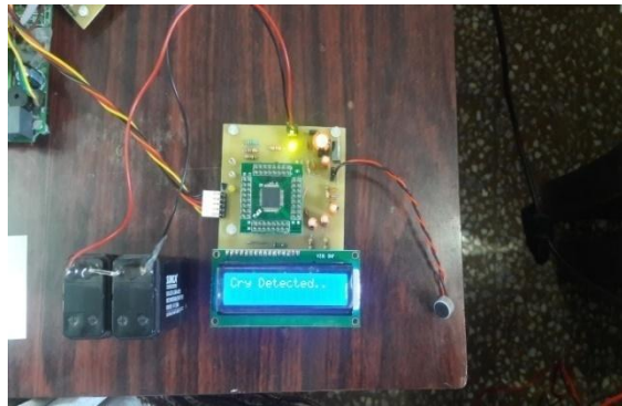
Figure 11: LCD showing detection of cry sound
