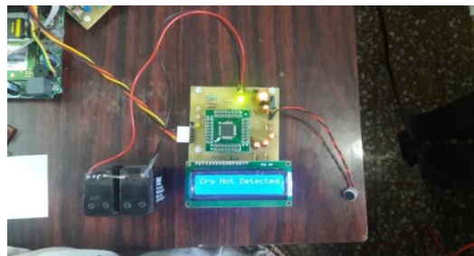
Figure 12: LCD showing cry not detected.
